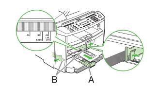
Slide the paper guide rail (A), and then pinch and slide the side paper guides (B) to match the size of paper.
